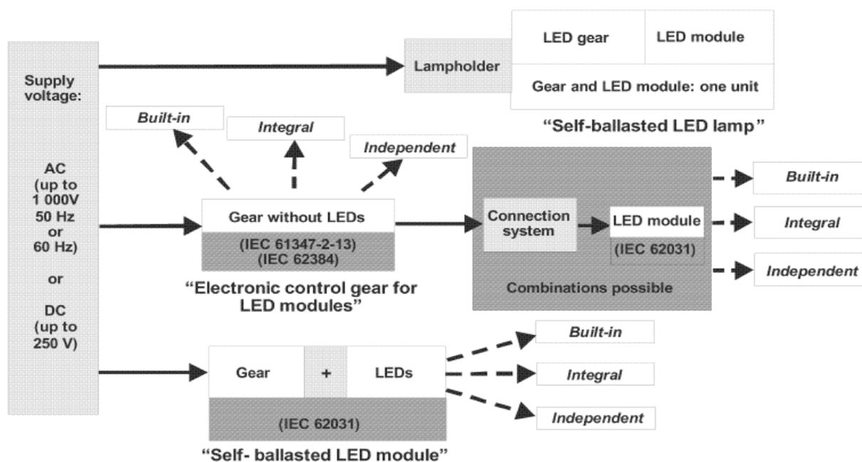
Figure 3 IEC 62031- LED module
