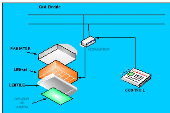
Figure 1 Solid state light with LED system
